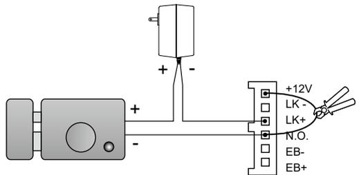
set to Normally Open on the Unlock Relay mode (default)
