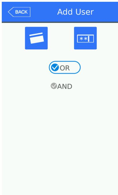
Select the Auth Type icon to change the authentication type of the user. If only card is registered, only a card icon will appear the same as password. If both are registered you can select a combination of both types using OR and AND.
